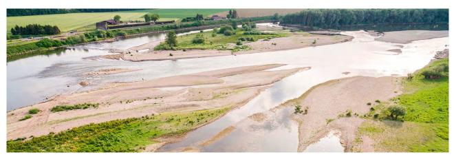
Restoration of the gravel pit area on the Flemish side with lowering of the river banks, and guiding the floods through channels
